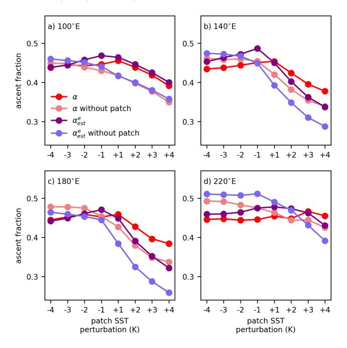
Figure S2. As for Figure 1 in the main text, but here including results for ascent fraction calculated with vertical velocity at 500 hPa (peach lines) and the entrainment-adjusted instability index (light blue lines) excluding directly warmed grid points (as defined as gridpoints with an SST change of greater than +0.4 K in the +4 K warming simulation).
